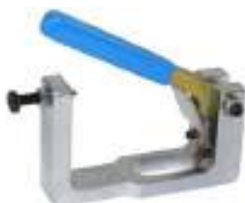
Engine Eccentric Shaft Fixture Holder Fixed for BM No.:114450 BMW N20 N26 N55
