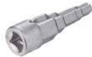
Radiator Spud Wrench Five Steps 10(3/8"), 7/16", 12.5(1/2"), 16 and 21mm. 12.5(1/2") Drive.
